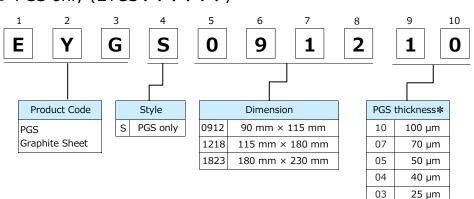
**\***PGS thickness of 17  $\mu$ m, 10  $\mu$ m does not than those above.
