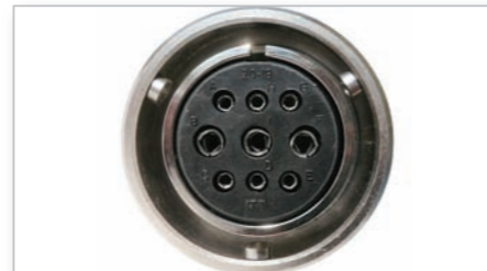
Cannon designed hard insulators are manufactured from high quality polyamide to withstand temperatures from -55C to +125C (-67F to +257F) and enable easy installing / uninstalling of contacts.
