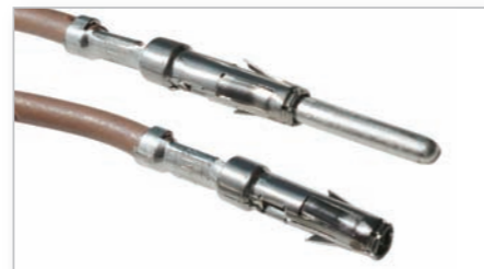
Tin (optional gold) plated Trident T2P stamped signal contacts accommodate wires from 0.14 to 2.5 mm 2 (AWG 26 - 14), perform up to 16 amps, and can be installed without any tools.
