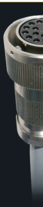
Legendary Cannon bayonet coupling design allows for fast and easy mating and unmating. An audible sound and visual indication, realized by a color marked snap-in position indicator, offer additional coupling security and vibration resistance up to 20 g's.
