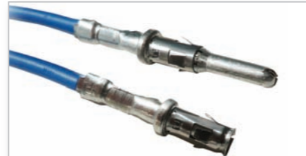
Tin (optional gold) plated APK25 stamped power contacts accommodate wires from 0.5 to 4.0 mm 2 (AWG 20 - 12), perform up to 30 amps, and can be installed without any tools.
